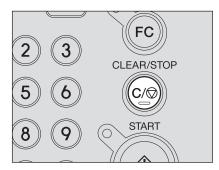
Scanning or copying stops. Press the [CLEAR/STOP] button again to end the copy job.
